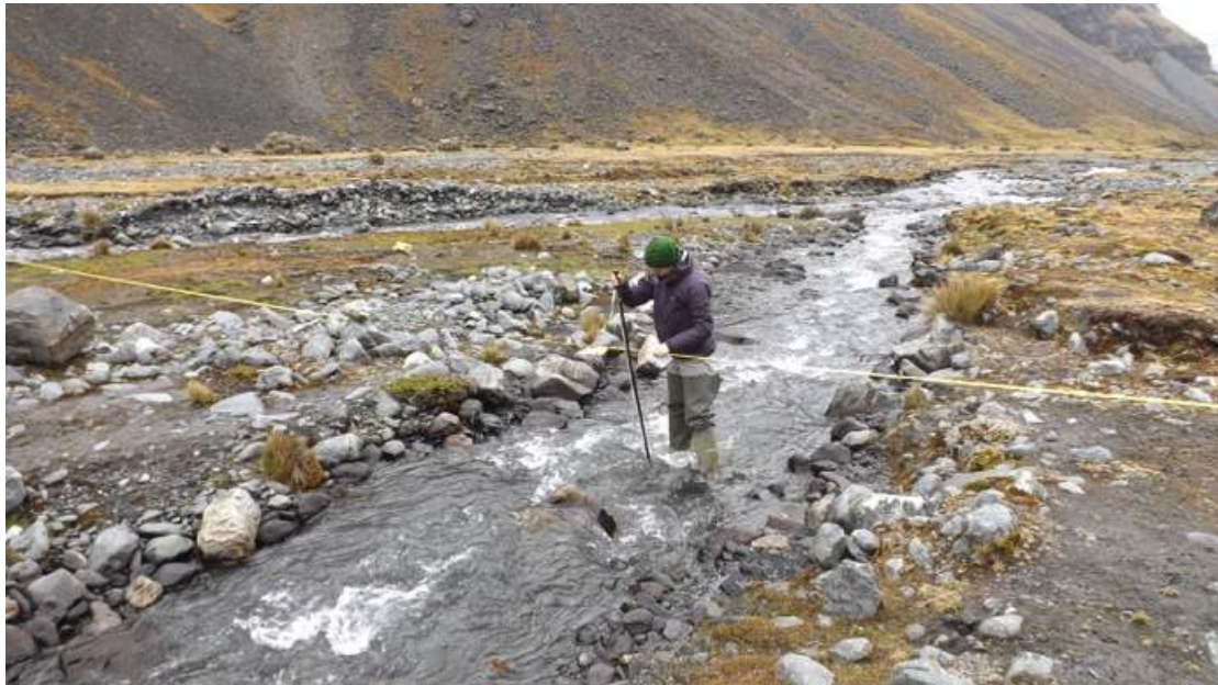
Figure 6 Measuring the stream and valley cross-section
